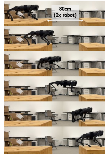
Fig. 5: Keyframes from a long jump (2x robot length)
