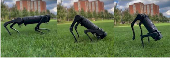
Fig. 6: Transition from quadrupedal walking to bipedal walking.
